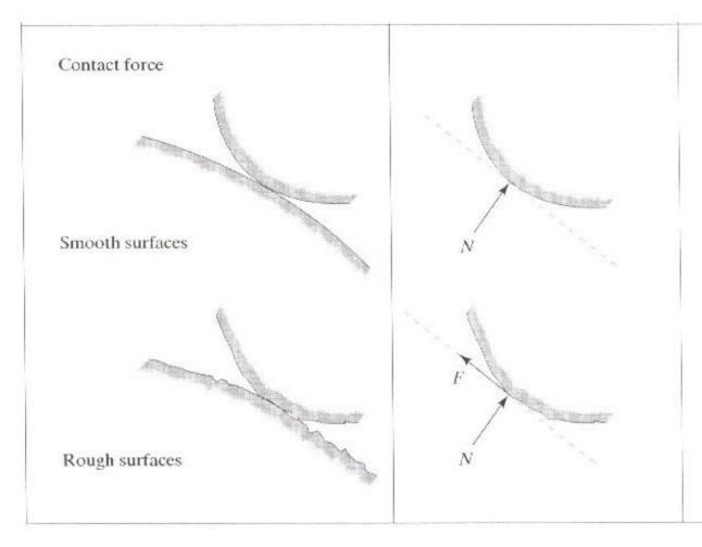
For smooth surfaces, the contact force, N, is toward the body, normal to the tangent drawn through the point of contact.
